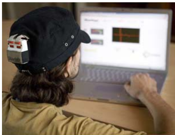
Figure 1: ENOBIO set in a cap for EEG recording. The data are transmitted wirelessly to the laptop.
