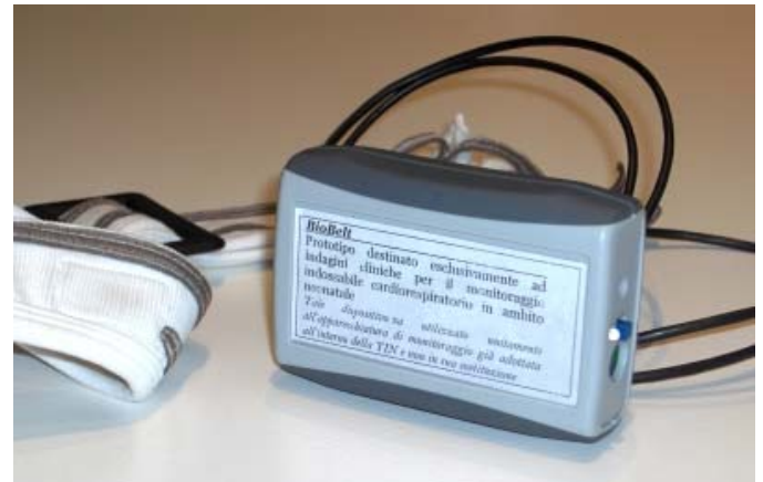
Fig. 2 The electronic unit for the monitoring: it includes the analog front-end the digital board for basic data processing and the BT transmission module.
