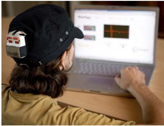
Fig. 1: ENOBIO sensor embedded in a cap. We can see the 4 channel inputs (red pins). In the picture, only two channels are plugged. The data are transmitted wirelessly to the laptop.
